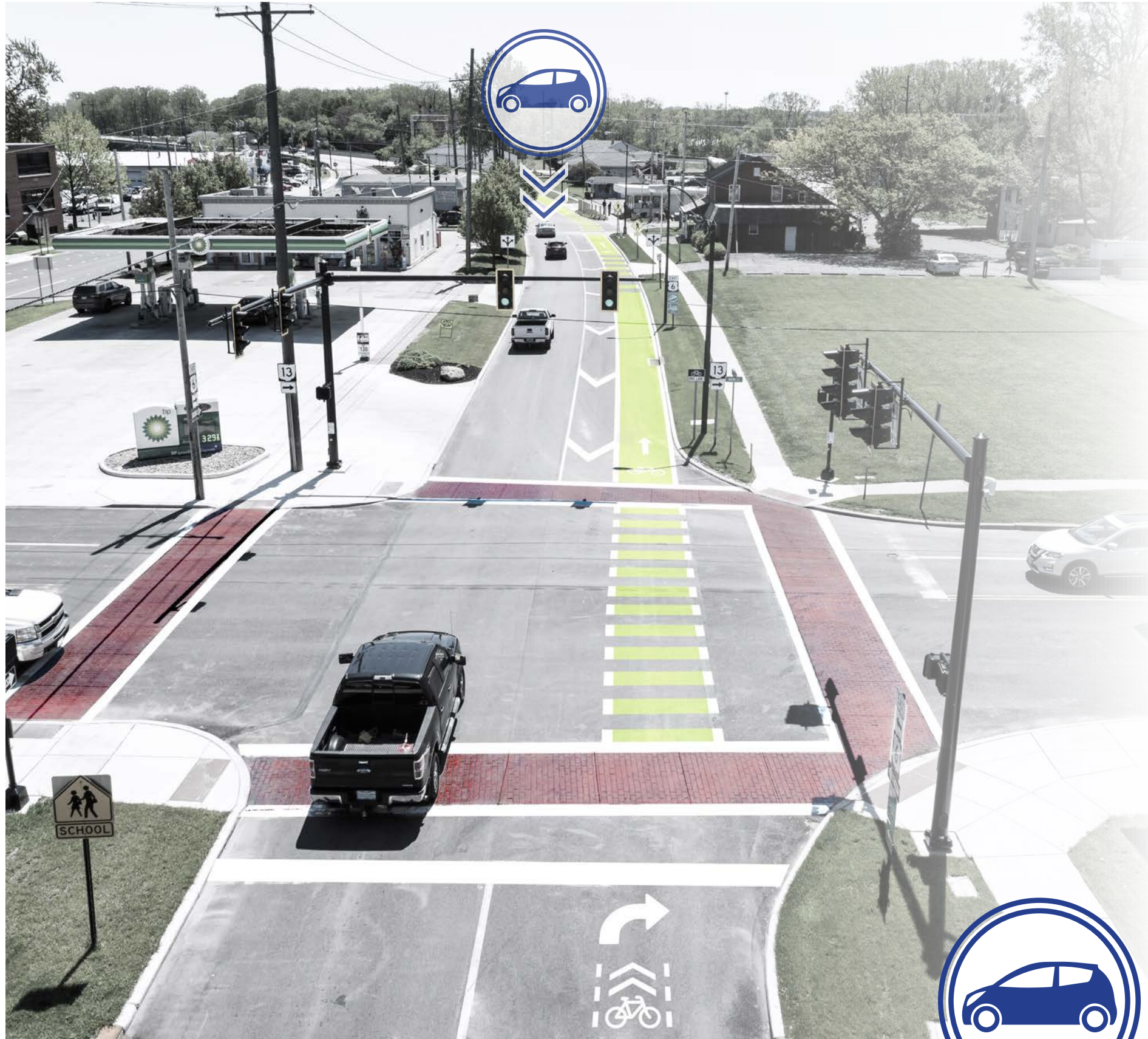
Painted bike lane delineation at Main St looking east. The view shows the updated shared bike lane and bike striping through intersections in relation to crosswalks.
