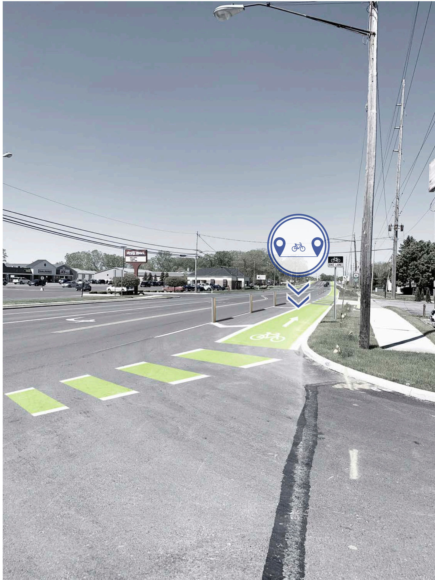
Painted striping to indicate delineation of separate protected bike lane from motorist traffic at the intersection of Berlin Rd - view looking west toward Downtown
